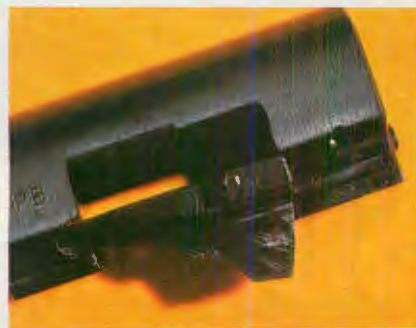
ABOVE: Full-open top of 92 SB slide eliminates malfunction from ejection port restriction. LEFT: Ambidextrous safety allows strong-or weak-hand use, right side view shows exposed ejector. RIGHT: Falling block lock assembly shows debt to Walther P-38. LOWER LEFT: Lever to
